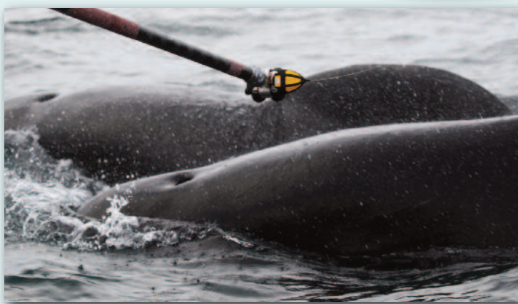
For smaller, faster species like the pilot whale, a hand-held pole is used to deploy the DTAGs. Tags need to be placed high on the back so that researchers can track the whale using the VHF signals given off by the tag when at the surface.
